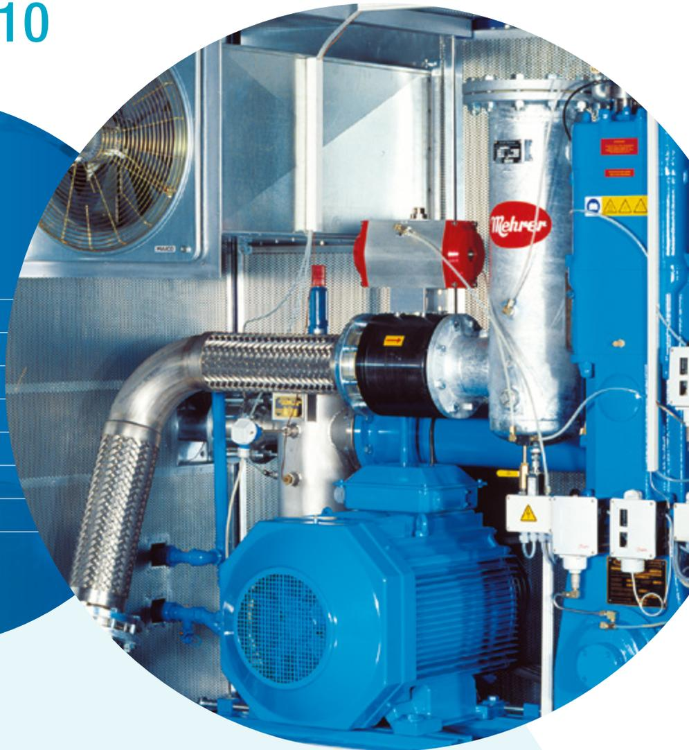
TEW 90 and TEW 110 are single-stage, water-cooled compressors. These products are used in the sectors Food & Beverage as well as Machine Construction and are developed for all oil- and silicone-free applications. Mehrer's vertical compressor design is space saving. The TEW 90 and TEW 110 can be operated with pre-pressure and frequency controlled working speed.
