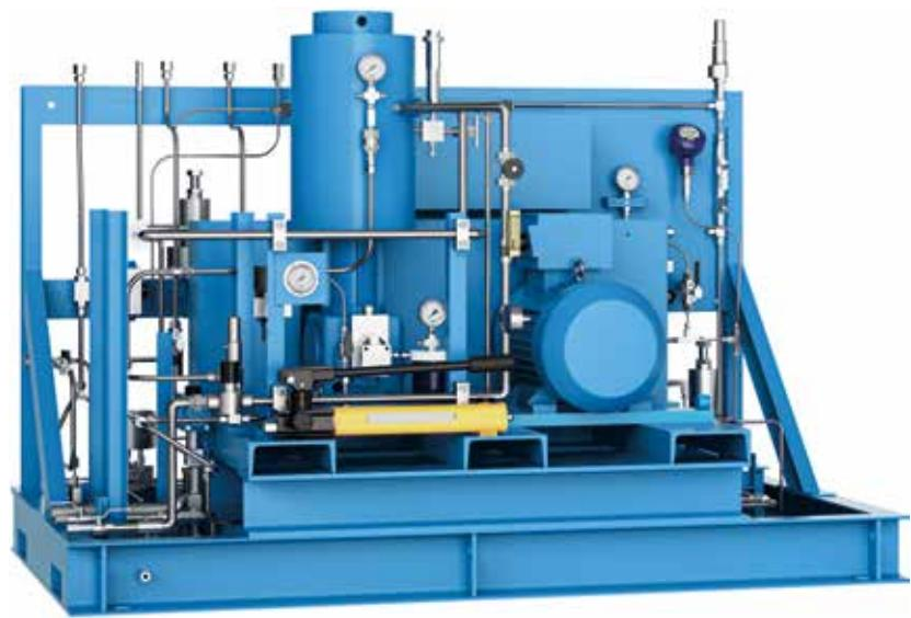
**Fig. 3:** Oil and leak-free high-pressure hydrogen compressor with suction pressures of 30 to 100 bar and a discharge pressure of up to 850 bar
