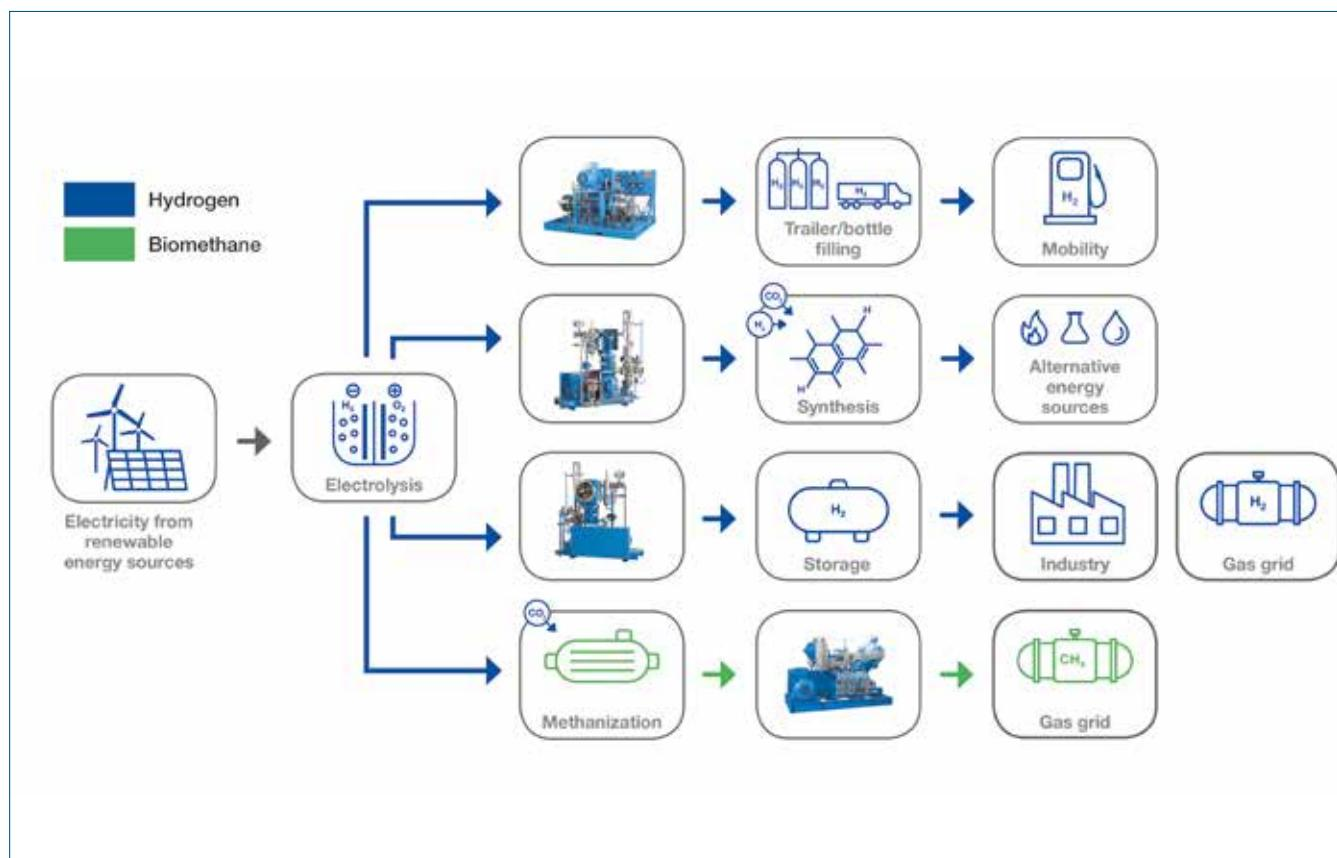
Fig. 1: The different production processes and end applications of hydrogen become special challenges for the compressor technology used
