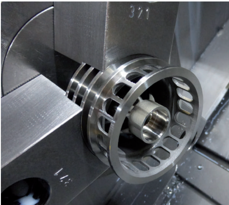
Fig. 4: Piston workpiece made by additive manufacturing undergoing machining of the piston ring grooves and the guide ring groove
