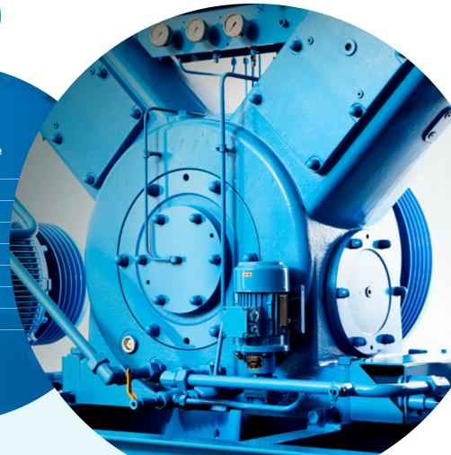
Compressors in the TVx 900 model series are available in single-, two- and three-stage designs. A booster version is also available in this series. Compressors in this series are used in the process gas industry. They are developed to compress technically complex gases reliably.
